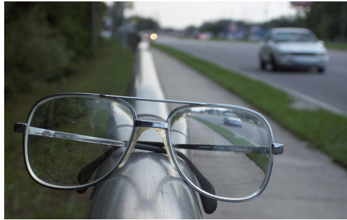
Figure 25.38 A car viewed through a concave or diverging lens looks upright. This is a case 3 image. (credit: Daniel Oines, Flickr)
