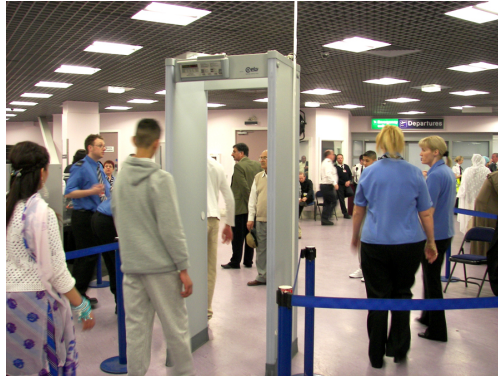
Figure 23.43 The familiar security gate at an airport can not only detect metals but also indicate their approximate height above the floor. (credit: Alexbuidrs, Wikimedia Commons)
