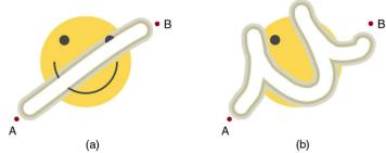
Figure 7.14 The amount of the happy face erased depends on the path taken by the eraser between points A and B, as does the work done against friction. Less work is done and less of the face is erased for the path in (a) than for the path in (b). The force here is friction, and most of the work goes into thermal energy that subsequently leaves the system (the happy face plus the eraser). The energy expended cannot be fully recovered.
