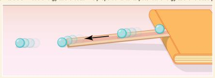
Figure 7.9 A marble rolls down a ruler, and its speed on the level surface is measured.
