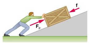
Figure 7.16 A person pushes a crate up a ramp, doing work on the crate. Friction and gravitational force (not shown) also do work on the crate; both forces oppose the person's push. As the crate is pushed up the ramp, it gains mechanical energy, implying that the work done by the person is greater than the work done by friction.
