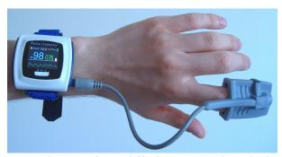
Figure 7.27 A pulse oxymeter is an apparatus that measures the amount of oxygen in blood. Oxymeters can be used to determine a person's metabolic rate, which is the rate at which food energy is converted to another form. Such measurements can indicate the level of athletic conditioning as well as certain medical problems. (credit: UusiAjaja, Wikimedia Commons)
