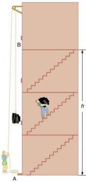
Figure 7.6 The change in gravitational potential energy  $(\Delta PE_g)$  between points A and B is independent of the path.  $\Delta PE_g = mgh$  for any path between the two points. Gravity is one of a small class of forces where the work done by or against the force depends only on the starting and ending points, not on the path between them.
