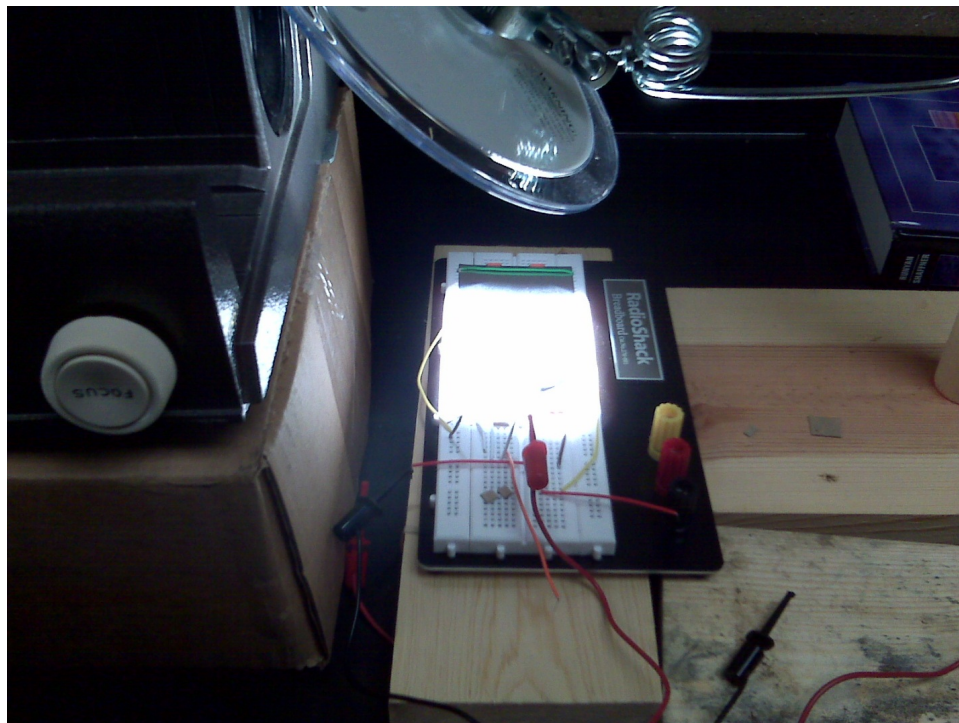
Figure 9.6: The picture shows the relative brightness of the light beam at an approximate intensity of 1000 \text{ W/m}^2 . A small concave mirror serves to both turn the beam and to concentrate it a small amount to reach that level.
