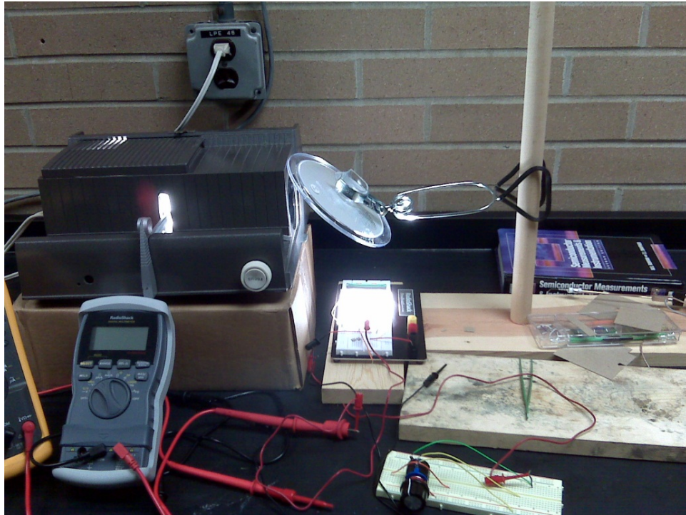
Figure 9.4: Test setup using a slide projector.
