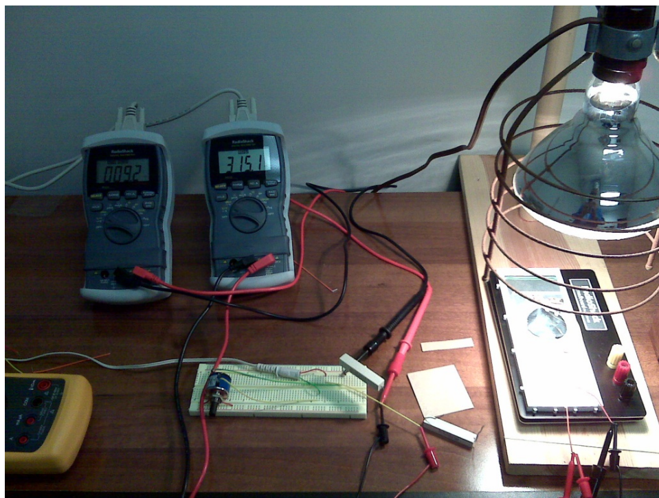
Figure 9.2: Simple test apparatus for qualitative measurement of the current-voltage output from an experimental thin film solar cell.
