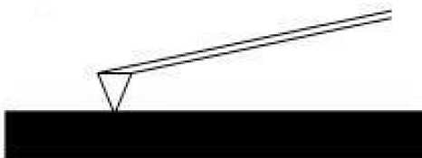
Figure 3.148: Schematic diagram of probe and surface interaction in contact mode.
