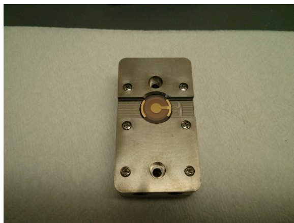
Figure 3.52: Correct position of the sensor in the chamber.
