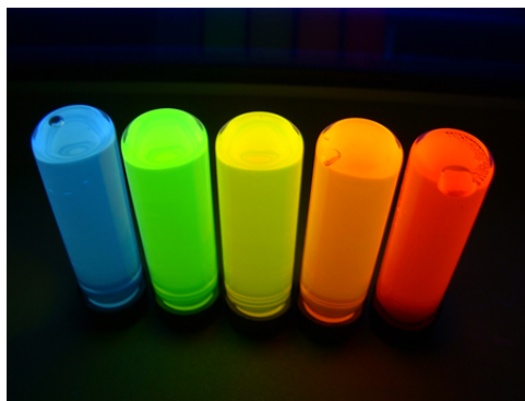
Figure 3.56: Fluorescing CdSe quantum dots synthesized in a heat transfer liquid of different sizes (M. S. Wong, Rice University).
