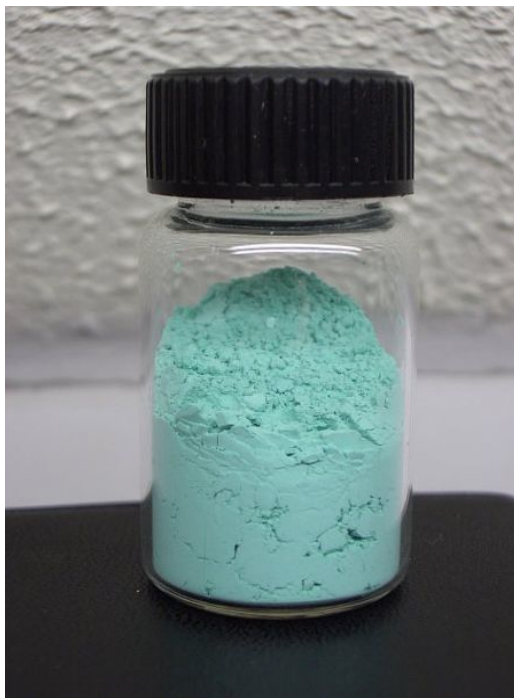
Figure 2.1: A sample of copper carbonate basic, \text{CuCO}_3 \cdot \text{Cu}(\text{OH})_2 illustrating the blue-green color.
