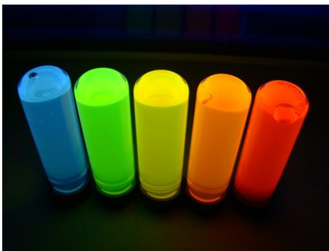
**Figure 7.44:** Fluorescing CdSe quantum dots synthesized in a heat transfer liquid of different sizes (M. S. Wong, Rice University).
