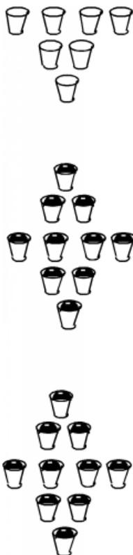
**Figure 1.4:** Silicon, with first two bands full and the next empty.
